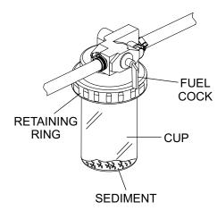
Figure 26. Fuel Water Separator
